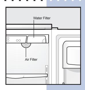
In general, you should change the air filter every six months to ensure optimal filtering of refrigerator odors. You may want to adjust this time period depending on the types and amounts of food you typically store in your refrigerator. To replace your air filter:
